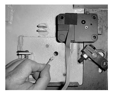
Once you've made sure the wire cable is not crimped or in contact with any sharp surface, attach the lock to the safe's mounting plate. Use the three 1/4-20 (or metric M6) screws provided. Tighten securely so the lock is attached firmly to the plate.
