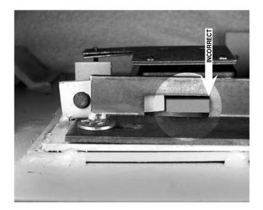
The boltwork bind has been relieved by removing a small amount of material from the right side of the boltwork opening. When the safe's boltwork is fully thrown to the locked position, there is an air space on all sides of the electronic lock's bolt.
