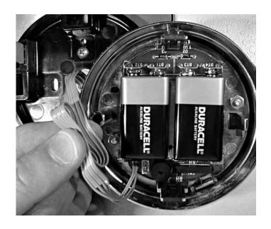
Place the keypad over the base. Make sure the wire cable is still clear of the three spring clips, then push the keypad firmly onto the base. It should snap into place. Note: To remove the keypad, pull the bottom (area nearest the S&G logo) away from the mounting base first.
