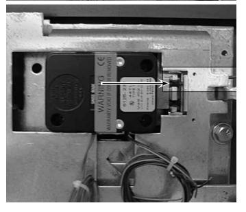
Note for safes with relock devices: Some installations require attachment of the safe manufacturer's relock device plate to the lock using the cover screws. If this is the case, be sure the thickness of the relock device plate(s) is not great enough to prevent the screws from engaging the lock case by <u>at least</u> four threads. If necessary, use longer 8-32 (M4) machine screws to ensure proper fit.
