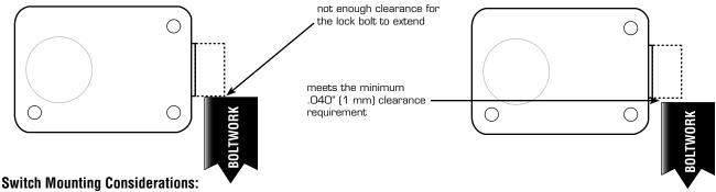
Location—Whenever possible, position the boltwork switch to sense the location of the cam plate or blocking bar that interacts directly with the lock bolt
